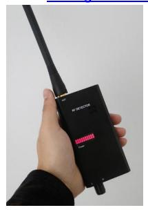
Cell phone Detector is to send the audio or video signal through electromagnetic waves. It is a machine designed to detect and fix the position of the hidden wireless tapping device.
